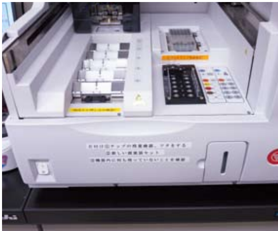
Precautions in the OSNA assay are pasted on the equipment to reduce human error.
