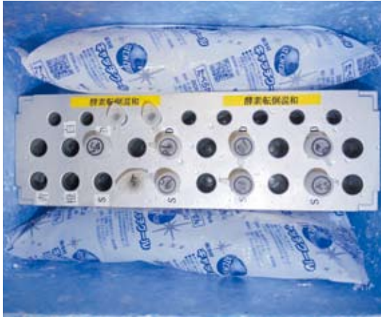
To prevent mix-up of samples and reagents, labels are pasted to indicate their pre-decided positions.
