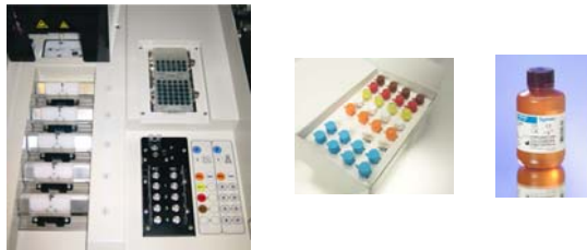
Figure 1: The OSNA system: view inside, reagent kit, and homogenising reagent (from left to right)
